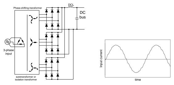
Figure 3. A 18-pulse rectifier power circuit and an input current waveform
