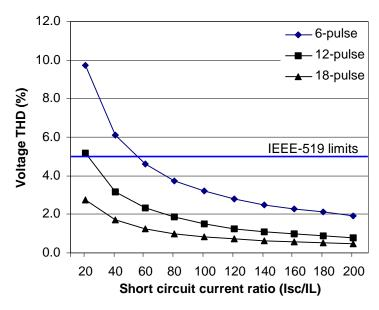
Note: Values in figures 6-7 may varies in figures 6-7 may vary depending on the power system environment. Figure 6. Input voltage THD according to rectifier type, the short circuit current ratio, and a 3% DC link choke.
