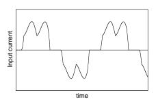
Figure 1. A 6-pulse rectifier power circuit and an input current waveform
