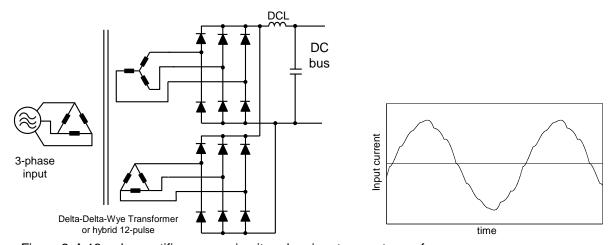
Figure 2. A 12-pulse rectifier power circuit and an input current waveform
